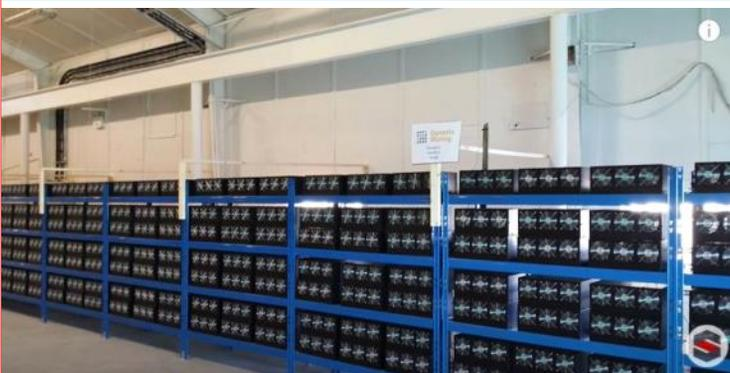
Application Specific Integrated Circuits - ASIC --> mining
